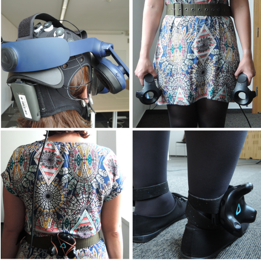
Figure 1. (Top left) Detail of EEG and HMD positioning, (Top right) Position of hand and waist tracking belt, (Bottom left) Position of waist tracking point, (Bottom right) Position of feet trackers
